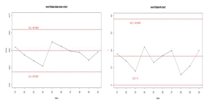
By the control charts of the new 10 thickness data, there are no points exceed the UCL and LCL, so we can know the process is in statistical control.
