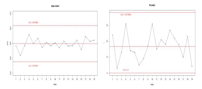
We can find that all the points are in between the UCL and LCL, the process is in-control.
