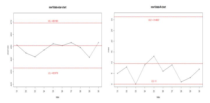
There is no point exceed the UCL and LCL, the process is in statistical control.
