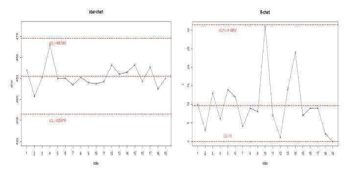
We can find that all the points are in between the UCL and LCL, the process is in-control.
